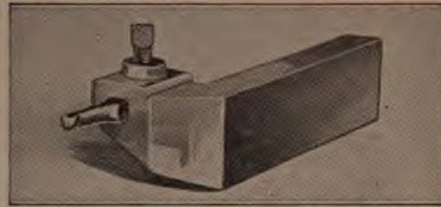
A Small Boring Tool, Formed from High-Speed Steel Stock by Grinding, without Forge Work, Is Convenient When Held in a Holder of This Design
